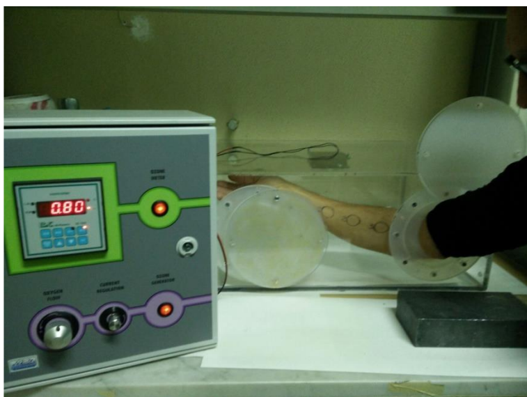
Fig. 2. The Ozone Exposure Chamber. The ozone generator, settled up to 0.8 ppm, was connected to a Plexiglass exposure chamber in a chemical hood.
